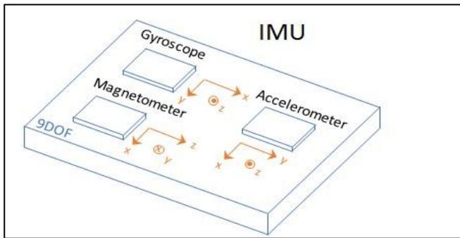
Figure 5.23 9DOF IMU
