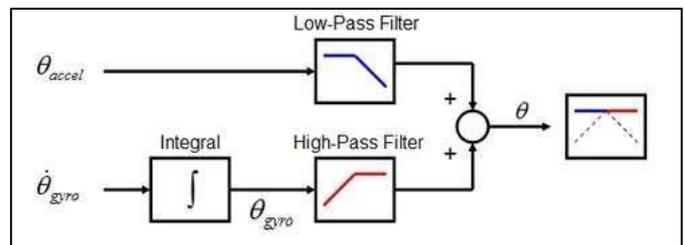
Figure 5.24 IMU Angular Velocity Calculation Process
