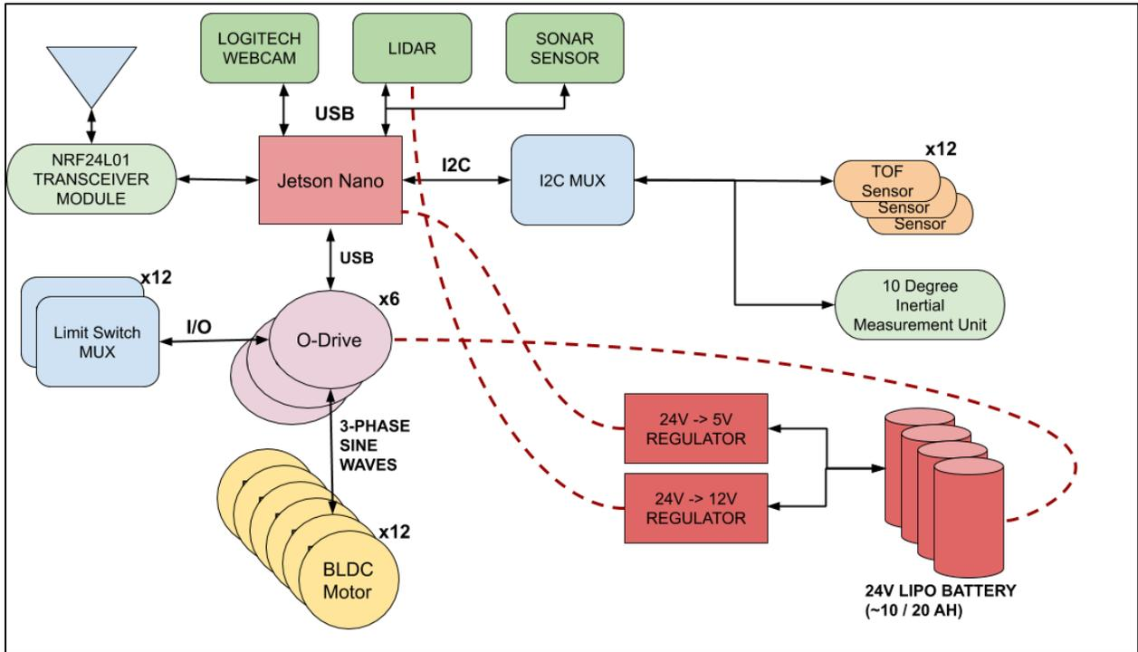
Figure B1.2. I2C MUX Block Diagram
