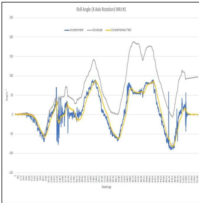
Figure 9.3 IMU #1 X-Axis Rotation Filtered versus Unfiltered
