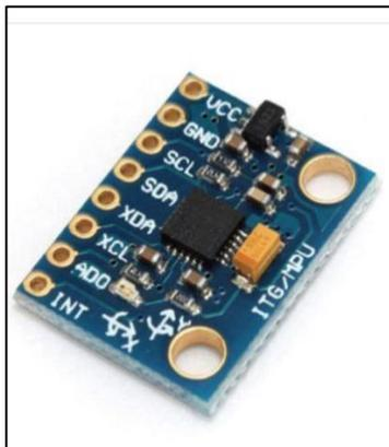
Figure 9.1 MPU6050 IMU
