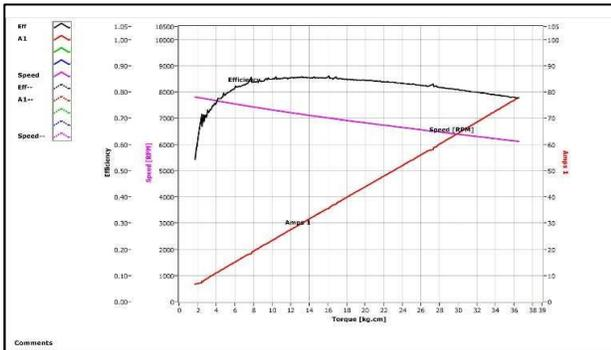
Figure 5.13 Turnigy Aerodrive SK3 Brushless DC Motor Efficiency: Rotational Accuracy Chart
