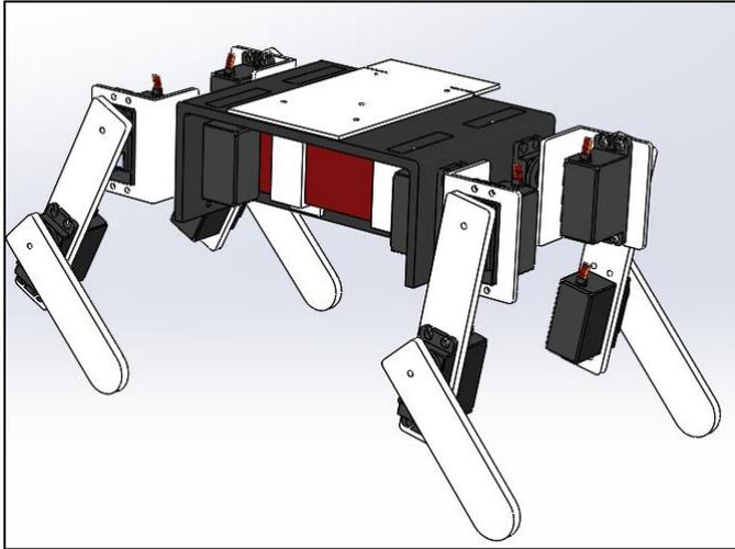
Figure 3.1 Small Scale CAD Model of Robotic Dog
