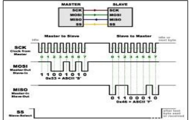
Figure 5.19 SPI Communication Protocol
