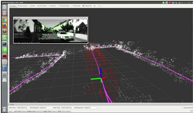
Figure 5.21 ORB-SLAM2 Point Cloud Map Example
