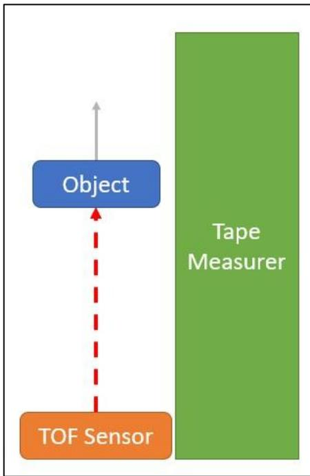
Figure 9.7 TOF Sensor Testing Procedure (Top-View)
