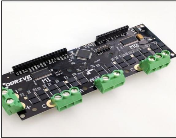
Figure 5.17 The ODrive Motor Controller v.3.5
