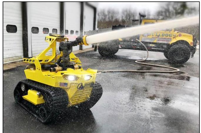
Figure 2.15. Thermite Fire Fighting Robot
