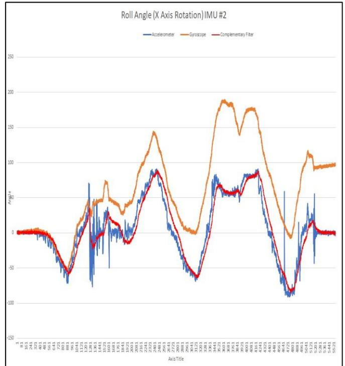
Figure 9.4 . IMU #2 X-Axis Rotation Filtered versus Unfiltered
