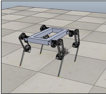
Figure 5.3 Diagram representation of our 12 Servo Dog
