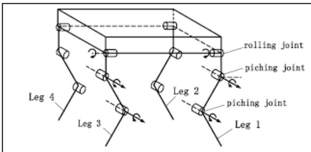
Figure 3.2 Small Model Joint Placement Diagram
