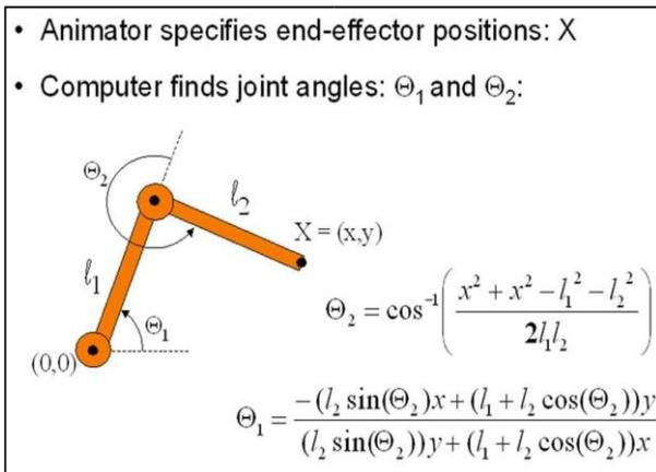
Figure 5.8 2D Inverse Kinematic Nonlinear Equations
