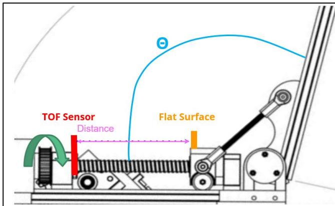
Figure 5.26 TOF Sensor Application
